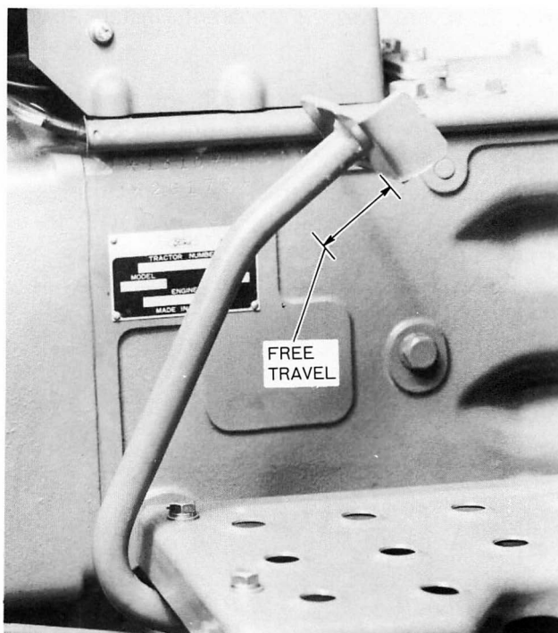
Figure 65 – Clutch Pedal Free Travel Adjustment
