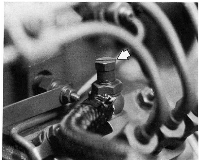
Figure 41 – Fuel System Bleed Screw
